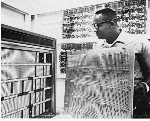
ANALOG PATCH PANEL which contains a program is held by Craig Jones (9422). This panel fits into the console of the EAI-680 analog computer (on the left). Other patch panels with programs are stacked in the background.
